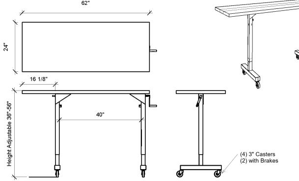
Designed to adjust to the height of the patient table during CRT implantation & extraction. Extension allows for RAO camera rotation without hitting the legs of the table.
